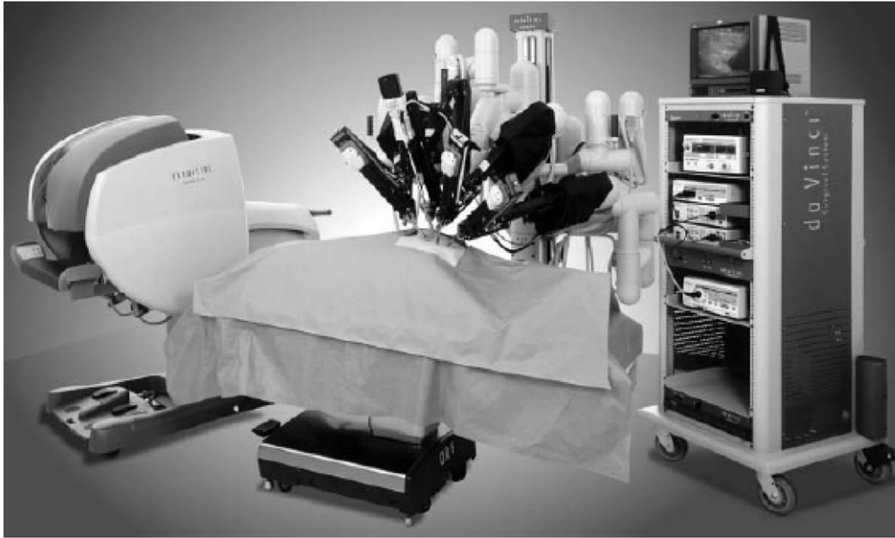
Figure 1 The Da Vinci robot (Intuitive Surgical™). The device consists of a master console (left) and a slave system (right) controlling 3 or 4 telerobotic arms. Photo courtesy of Intuitive Surgical (Sunnyvale, CA, USA).
